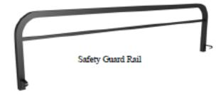
Safety guard rails are highly recommended for <u>ALL</u> spring heights. To attach the guard rail, slide the mattress so the guard rail can lay flat on the spring. Engage the two brackets of the guard rail to the spring and raise it to the vertical position. The mattress can now be repositioned and will hold the guard rail in its upright position.
